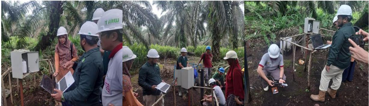
Gambar 38. Proses Pengecekan dan *Reinstall* Alat Perekam Kelembaban Tanah
