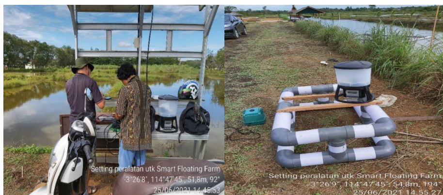
Gambar 29. Setting peralatan automatic fish feed, digital timer, dan aerator
